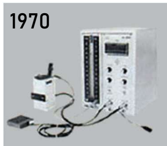
1970 First in Japan Rat tail artery pressure measuring device: A non-invasive device that can measure arterial pressure with a tail cuff.
