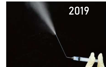
2019 First in Japan Endotracheal spray: possible to spray viruses and chemical solutions into the trachea so as not to burden animals such as mice and rats as much as possible.
